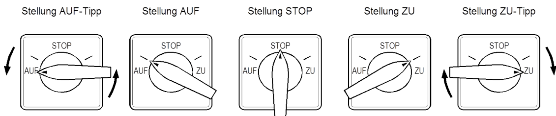
Figure 3: Control switch S31
